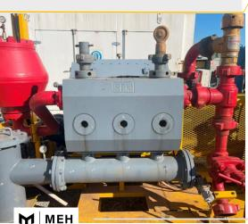
Powered by a CAT C32, the SPM TWS2250 is a proven performer that can deliver up to 850GPM @ 3000 PSI, all in a and highly mobile, jack-up configuration.
